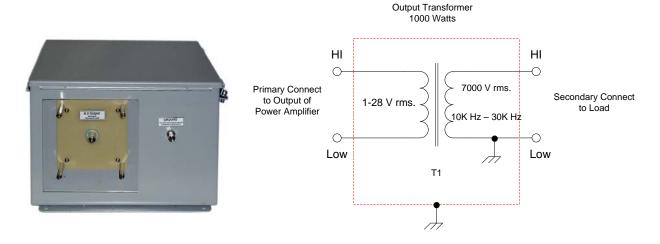
This model AL-T1000.6 high frequency high voltage output transformer was manufactured to meet the following basic specifications.
